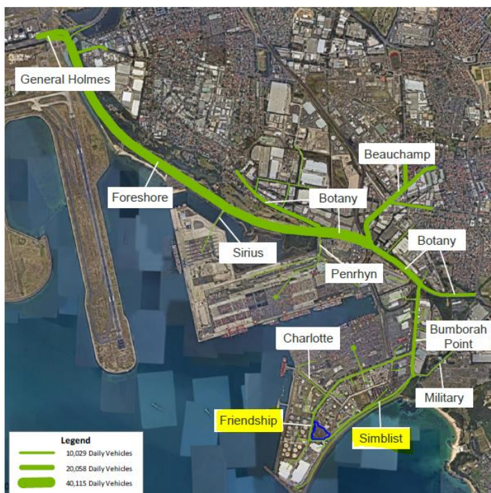
Figure 5: Average weekday total vehicles (with road labels) Source - File Port Botany Freight Study
